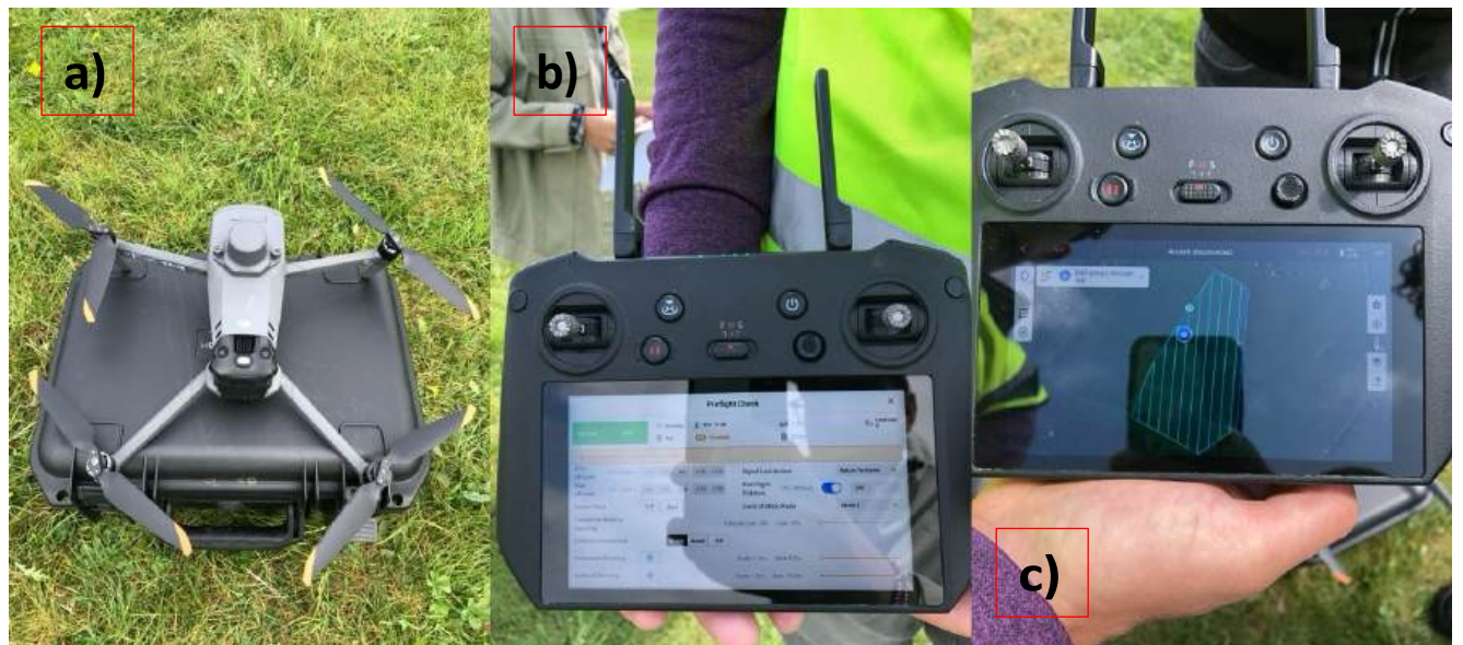
Figure 8: The merged images (a) show the DJI Mavic drone being calibrated prior to taking a flight (b) shows the ground transmitter assigning a mission flight path, height and speed to extract the data.
