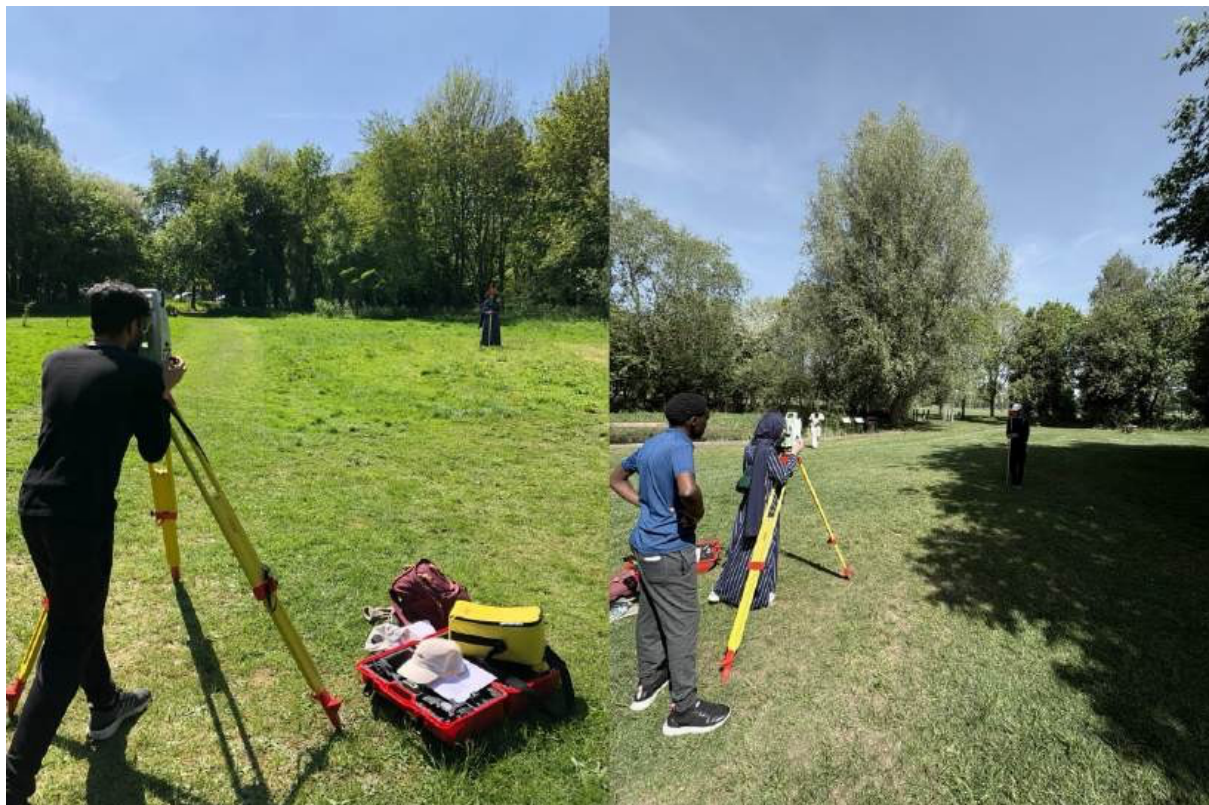
Figure 1: The two merged images show the total station equipment in action collecting elevation data points via transect method, where one person operates the instrument and another holds the prism pole and walk towards the instrument.
